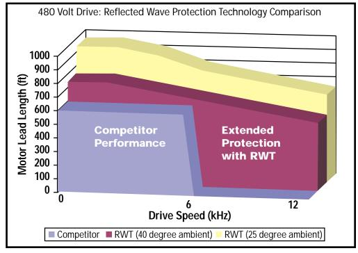
The RWT protects motors from reflected waves at frequencies up to 12 kHz, a far greater range than other devices.
