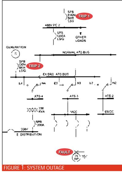
existing 30 year-old facility. A power system study performed on the new electrical distribution system, only assured coordination between protective devices within the new system. The new electrical system consisted of a 4160V switchgear, 4160V primary/480V secondary substations, 480V and 208V panelboards and 480V and 208V motor control centers (MCC).
